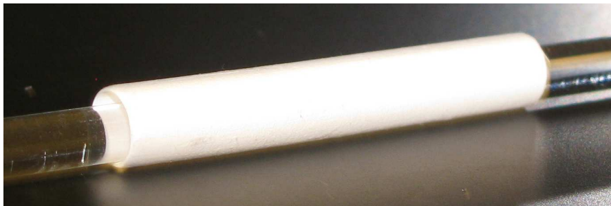
Figure 2-7. PCL tubular construct prepared by electrospinning.
